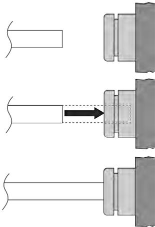
To connect the exhaust line to the exhaust port's PTC fitting, firmly push the appropriate tubing into the hole in the center of the connector until it seats in the connector. Refer to the figures at the left.
